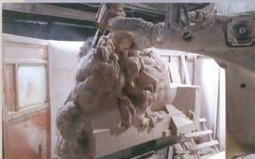
One of the lions being worked on the robot at Stoneworld (above) and being finished by hand at Chichester Stoneworks (below).
